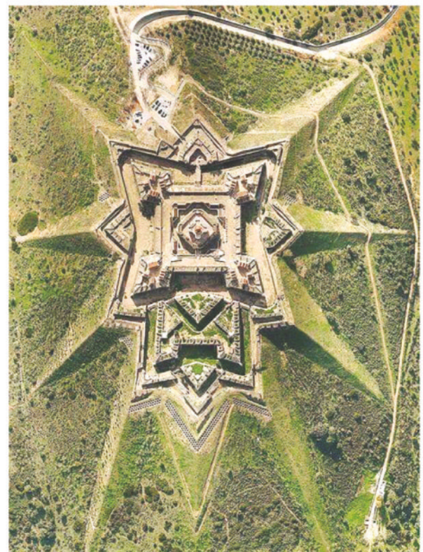
Inspiring example of star fort and horn work, Aerial photo of Our Lady of Grace Fortress, Elvas, Portugal.
